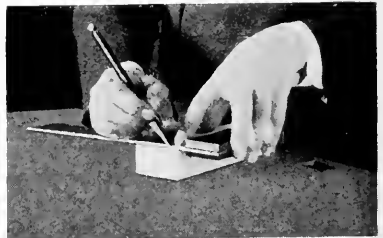
Fig. 3. Squaring the End with Try Square and Pencil.
